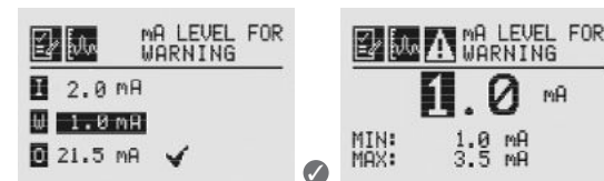
Figure 13. Set mA Levels for Warning
