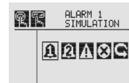
Figure 16. Alarm/Fault Simulation Menu
