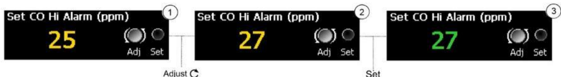
Figure 22 Example of alarm set-point adjustment
